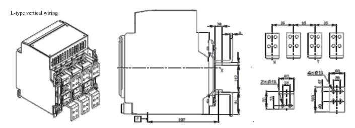
Note: For the 3-pole circuit breaker, X and Y are the symmetric axes of the front cover;
