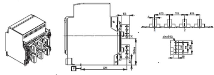
Note: For the 3-pole circuit breaker, X and Y are the symmetric axes of the front cover;
