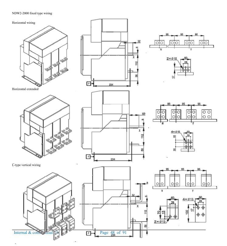
Note: For the 3-pole circuit breaker, X and Y are the symmetric axes of the front cover;
