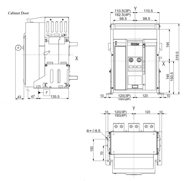
Note: 3-pole breakers X and Y are front cover symmetry axes;
