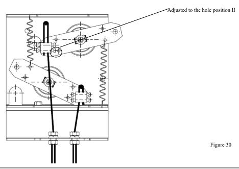
lacktriangleThree interlocking cables
