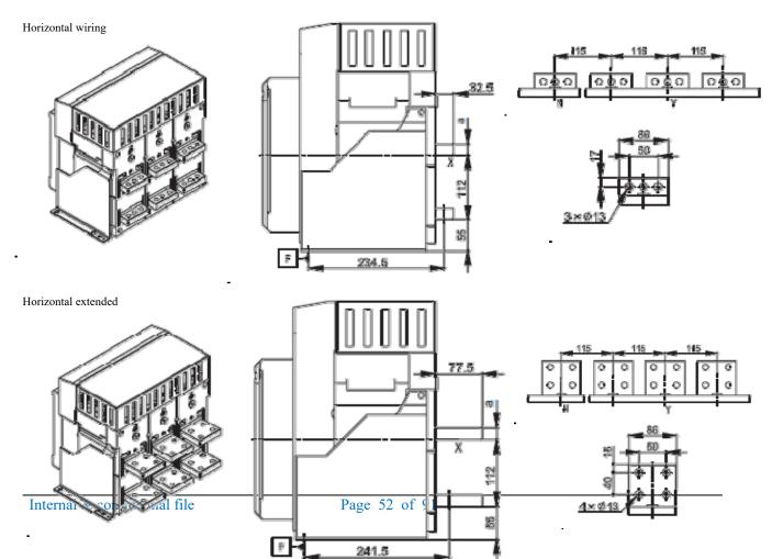
Note: For the 3-pole circuit breaker, X and Y are the symmetric axes of the front cover;
