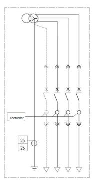
Leakage grounding protection
