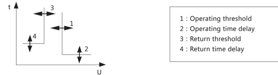
Figure 9 Overvoltage protection operating principle
