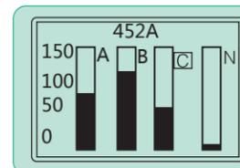
Control unit displays default interface when being powered on. To return to the default menu, press or button for relevant theme menu.
