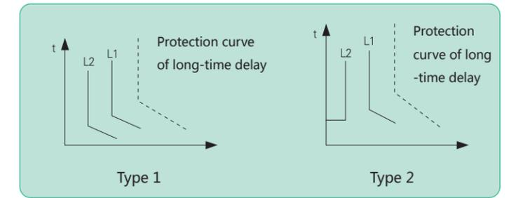
Figure 11 Operating characteristic of load monitoring on current
