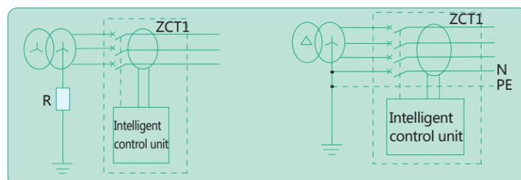
Figure 5 Detection schematic of leakage protection
