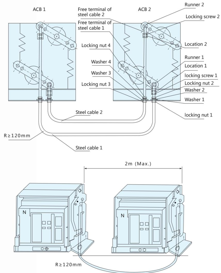
Connection Diagram of Connecting Rods Interlocking Between Two ACBs
