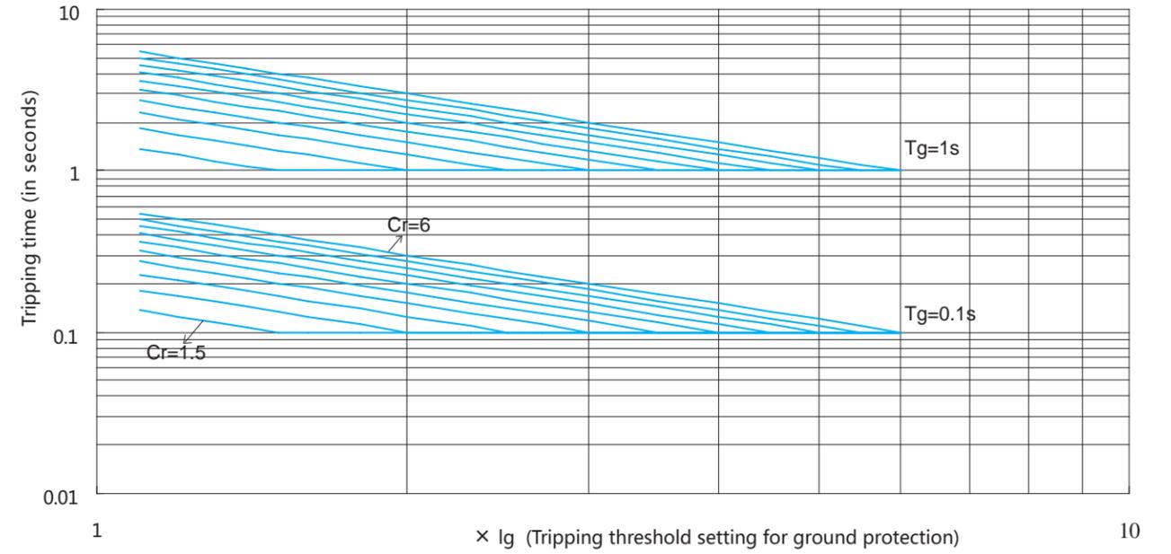
Figure g2. Leakage Protection
