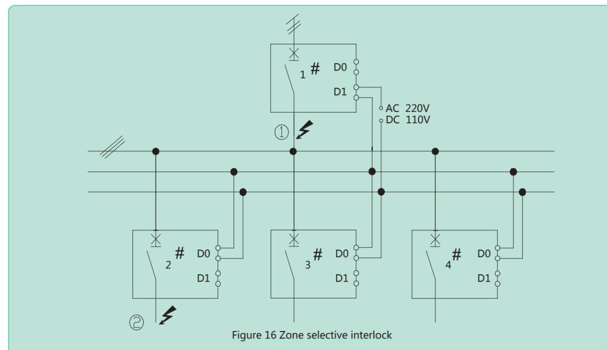
Zone selective interlock includes short-circuit interlock and grounding interlock. Among two or more levels associated ACBs in one power system:
