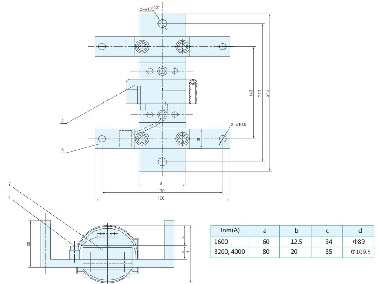
1 - Wiring board 2 - Bus 3 - Fixed plate 4 - Transformer
