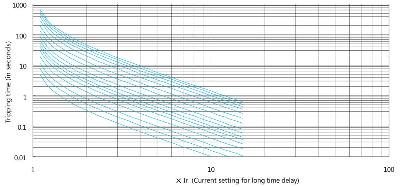
Figure S4. Inverse short-time delay - Extremely inverse time (for motor protection)
