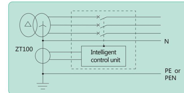
Figure 4 Detection principle of differential value type ground protection
