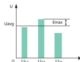
Figure 14 Voltage unbalance
