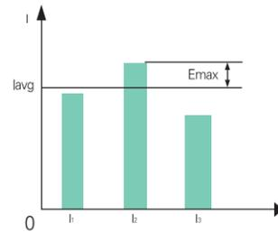
Figure 7 Current unbalance protection
