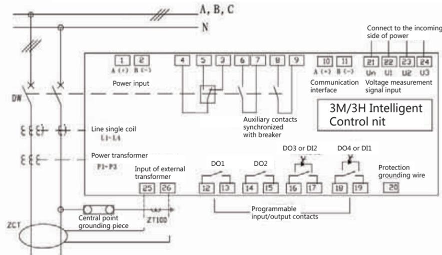
Diagram 19 3M/3H Input and output interface
