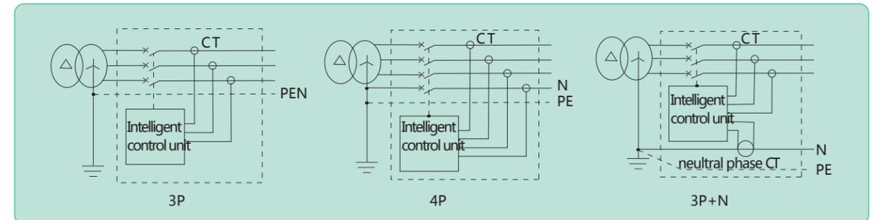
Figure 3 Detection principle of differential value type ground protection
