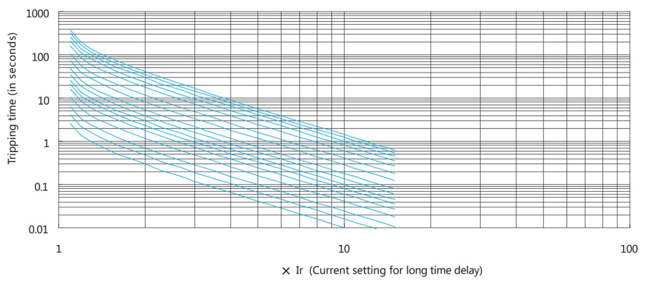
Figure S5. Inverse short-time delay - High voltage fuse compatible
