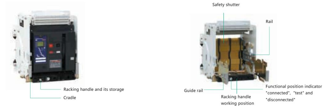
Drawout ACB is comprised of breaker itself and cradle. There are rails on both two side of cradle, with which guide rails are equipped. Drawout ACB connects the main circuit by plugging the bus of the breaker into the bridge shaped contacts in the cradle.
