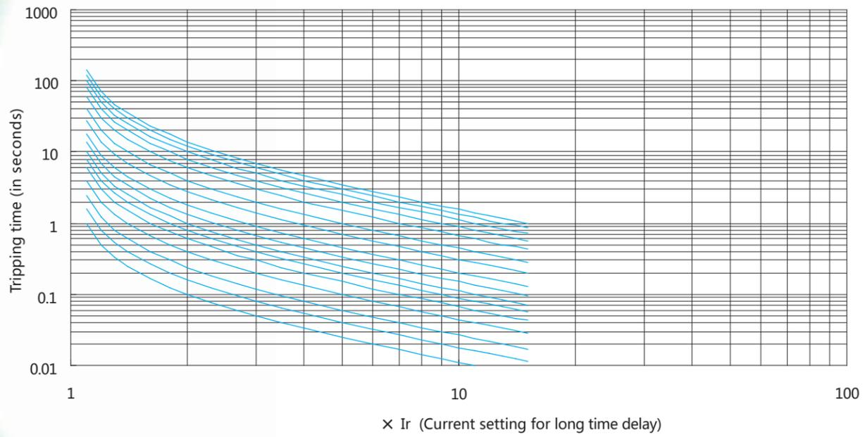
Figure S3. Inverse short-time delay - Extremely inverse time (for general power distribution protection)
