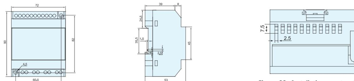
Figure 22 Installation construction of ST201, ST power module (IV)
