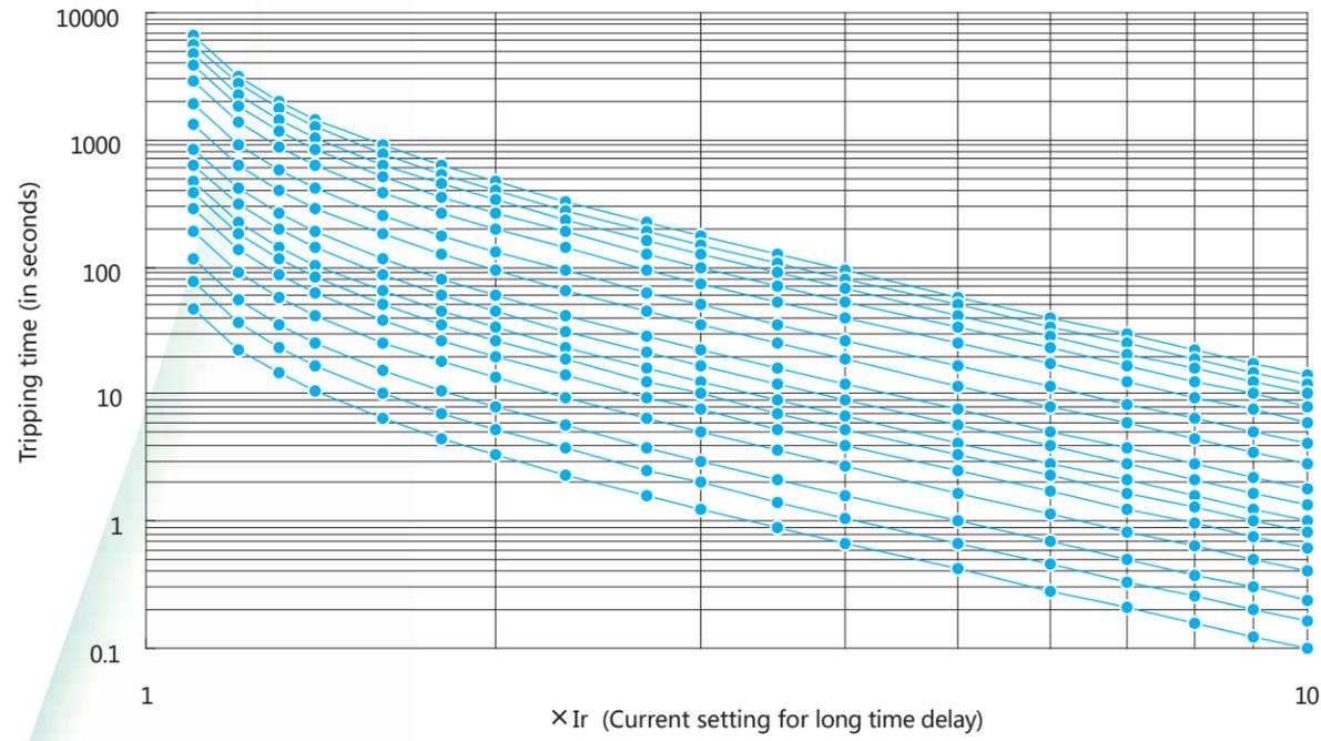
Figure A5. Extremely inverse time (For motor protection)
