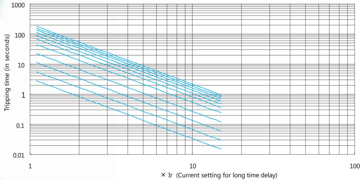
App. C Tripping Curves for Ground/Leakage Protection
