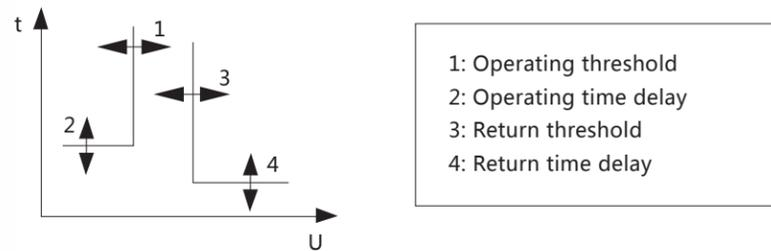
Figure 8 Undervoltage protection operating principle
